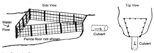
Figure 2. Culvert Protective Fence.
