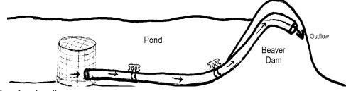
Figure 3. Pond Leveler pipe diagram.
